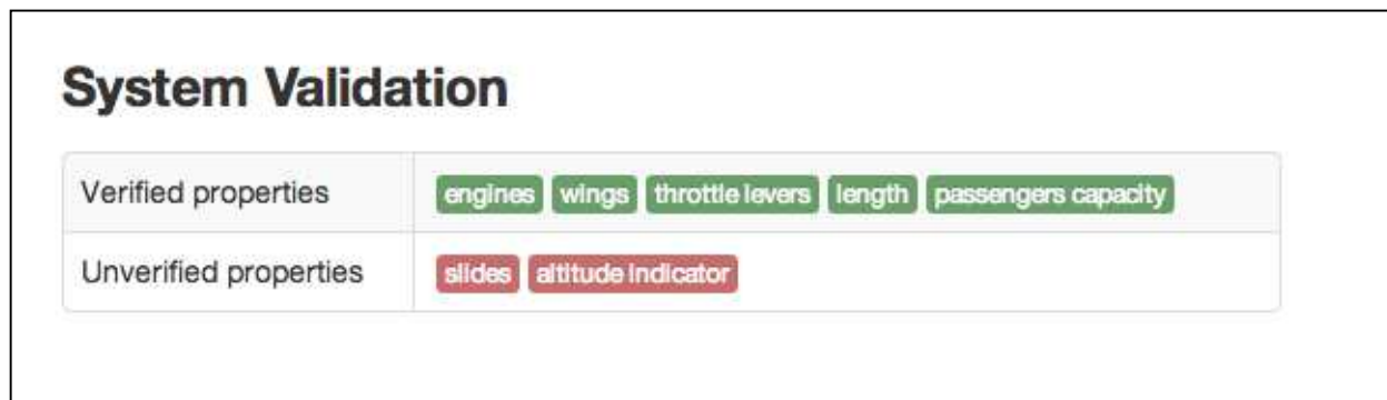
Figure 15. This is the final output from the application workflow. It shows what properties are verified (i.e., are present in the system requirements) and which ones are not.
