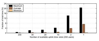
Fig. 8. Percentage of total time BER target is not met by a user as a function of number of available uplink time-slots (200 users)
