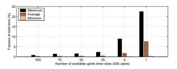
Fig. 9. Percentage of total time BER target is not met by a user as a function of number of available uplink time-slots (500 users)
