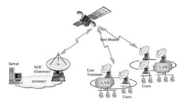
Fig. 1. Satellite communication system architecture. The satellite provides broadband access to users across multiple spot-beam locations.
