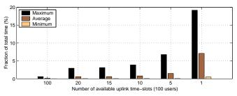
Fig. 7. Percentage of total time BER target is not met by a user as a function of number of available uplink time-slots (100 users)
