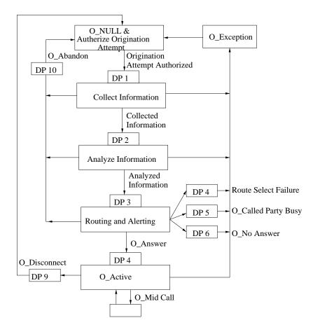
Figure 2.6: Originating BCSM for CS1
