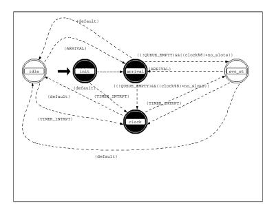
Figure 4.10: State diagram for the mobile queuing system
