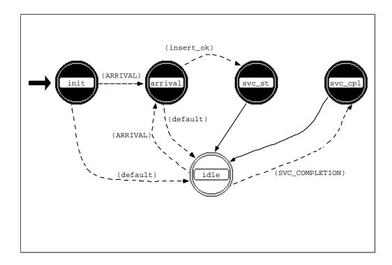
Figure 4.2: State diagram for the base station queue
