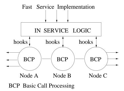
Figure 2.2: Typical IN service processing model
