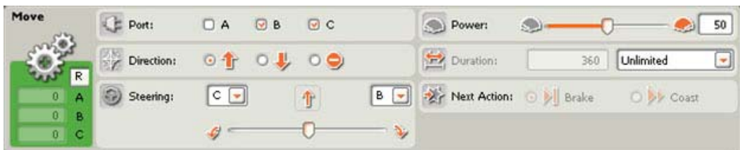
Fig.10 Description of move block
