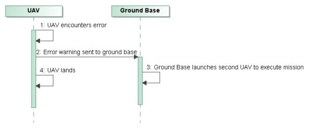
Figure 13: UAV Error Sequence Diagram
