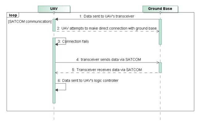
Figure 12: SATCOM Communication Sequence Diagram
