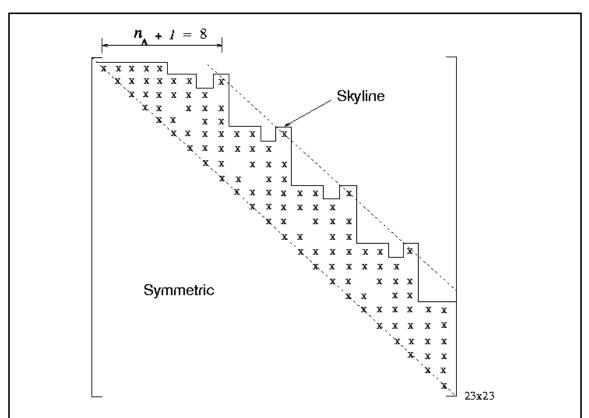
Figure 4.4: The structure of the system matrix  $A^t$  of our physics-based fish model, the skyline of  $A^t$  and its half-bandwidth  $n_A$ . Each "x" represents a non-zero entries.
