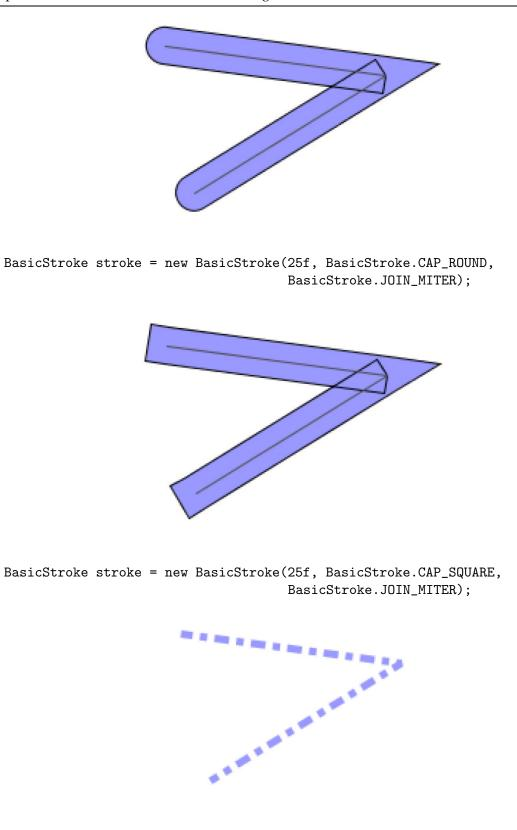
BasicStroke stroke = new BasicStroke(5f, BasicStroke.CAP\_BUTT, BasicStroke.JOIN\_MITER, 1f, new float[] {10, 5, 5, 5}, 2);
