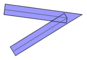
BasicStroke stroke = new BasicStroke(25f, BasicStroke.CAP\_BUTT, BasicStroke.JOIN\_MITER);
