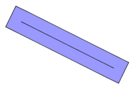
in user space. If the Graphics2D's transformation has been modified, it is applied to this figure and if the transformation results from a non-uniform scaling, then the thickness of a line will depend on the angle at which it is drawn. The interior of the region is then filled. In other words, draw is really just a special case of fill.
