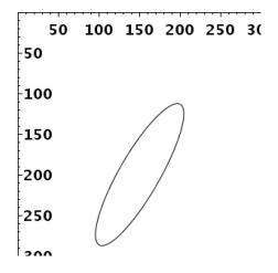
While the AffineTransform is created by first translating, then rotating and scaling, the effects on the circle occur in the opposite order: first it is scaled, then rotated and finally translated. This is natural given the order in which the transformations are composed.
