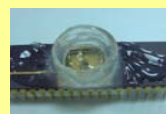
A Silicone Room Temperature Vulcanate isolates cells from toxic packaging and insulates exposed bond wires from cell medium.
