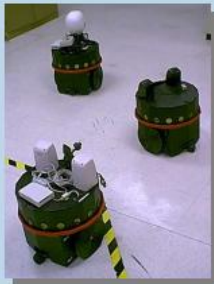
A test-bed for control, communication and sensing technique of use in Formation Control
