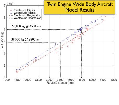
Airline data has much wider variability in fuel used because the data is taken from 79 distinct days Airline data supplied by Airlines for America
