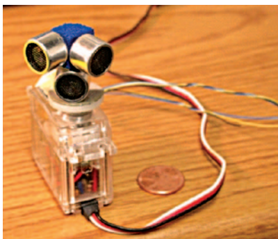
[FIG3] An example binaural sonar head with two ultrasonic microphones mounted on top, with an ultrasonic loudspeaker below. The assembly is shown mounted on a rotating platform.
