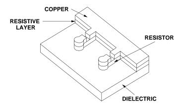
Figure 4: Embedded Resistor [21]
