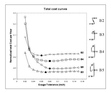
Figure 7: Total costs for the four design alternatives under varying gauge tolerance
