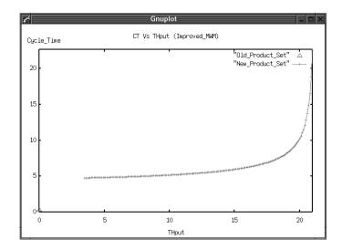
Figure 4: CT as a function of Throughput for New Product
