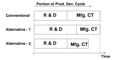
Figure 8: Lower manufacturing cycle time allows more time for research and development
