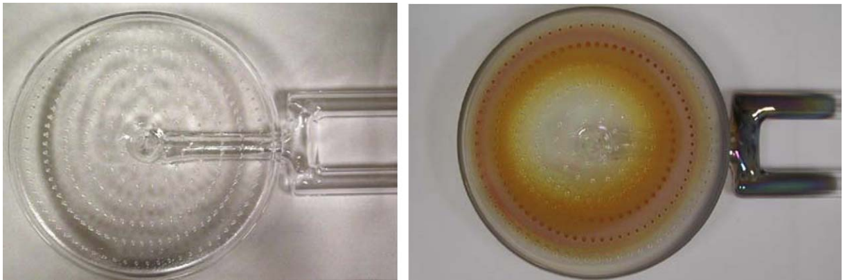
Fig. 3. Showerhead deposition pattern: before growth run (left) and after growth run (right).
